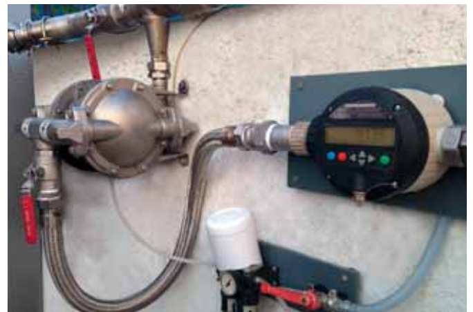
Shown in version for manual batching & totalizing being used with an air-operated double diaphragm pump.
