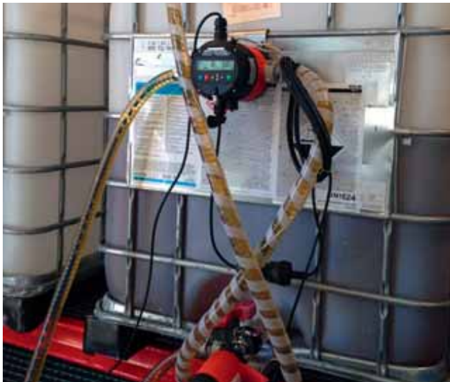
Shown in version for semi-automatic with one-touch start batch/metering ability utilizing bottom outlet of IBC.
