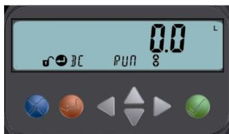
The FLUXTRONIC® is set to manual operation on delivery, it is now in display operation. This kind of mode is for manual filling, the quantity is shown at the display.
