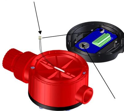
Open the battery compartment using an appropriate tool.
