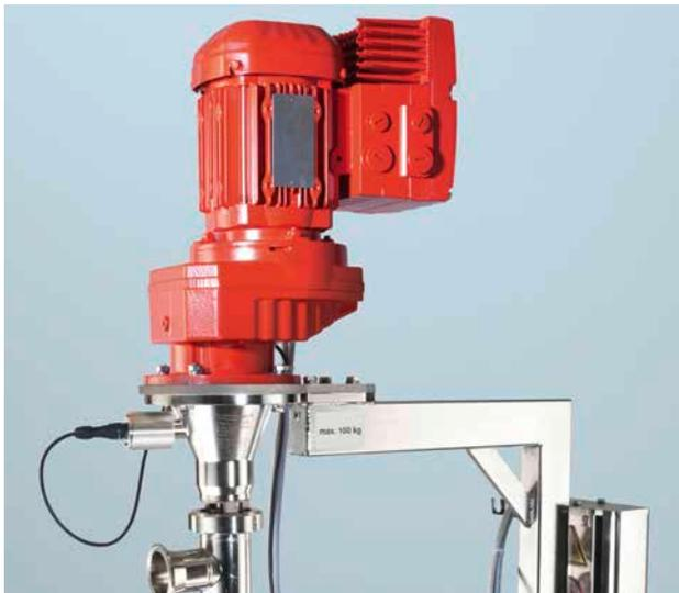
A pump with a impulse sensor is available for contact-free flow measurements.
