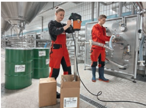
VISCOPOWER F 570 for pumping viscous concentrated fruit juice.
