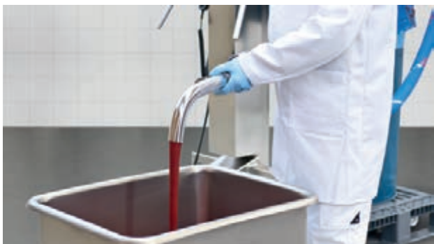
Basic food such as vegetable and fruit concentrates can be gently transferred with low-shear.
