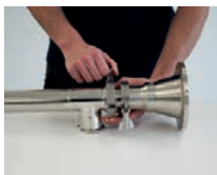
Open clamp on pump tube
