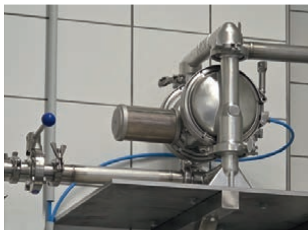
FLUX SD20 compressed air diaphragm pump in the Hygiene Design
